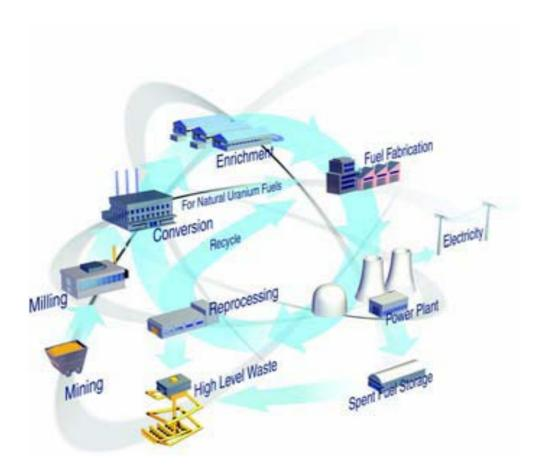
Schematic drawing of the nuclear fuel cycle<sup>3</sup>
